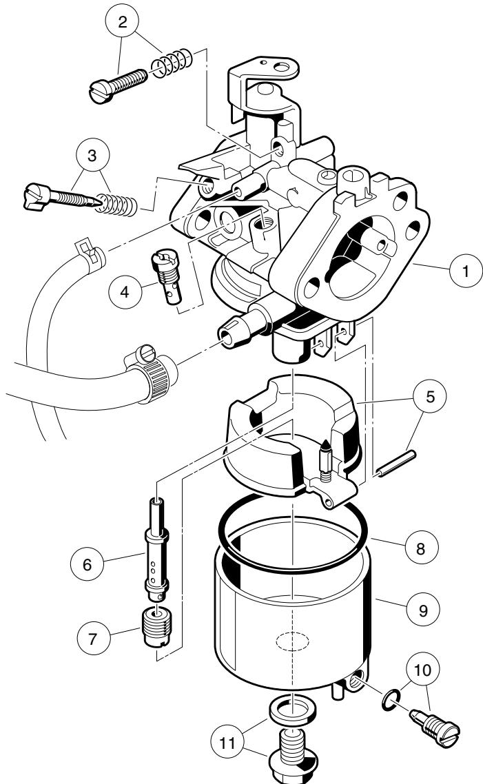
**CARBURETOR ASSEMBLY, FE350 ENGINE–
