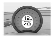
The service due notification will appear when the vehicle has reached the milage or hour limit. Please contact the nearst Garia dealership to get the service carried out accordingly.
