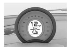
Critical battery level: This appears in cluster when the car has a minimum range left and can only drive in limp mode at 4 Mph / 6 Kph. The car urgently requires charging.
