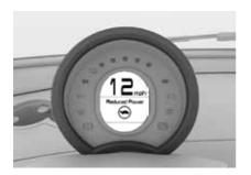
Reduce speed for a short period of time and the vehicle will return to normal operation.
