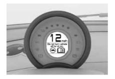
This message is important to respect, the vehicles requires a "cool down" period of 2 minutes, due to seriously heavy use. After two minutes the vehicle will return to normal operation. The reason for this function is to avoid overloading of important electrical components in the drive system.
