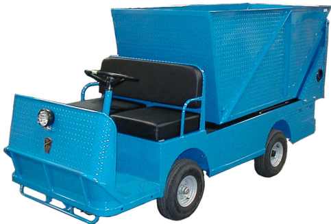
B 2-48-36 Equipped with optional hydraulic dump bed
