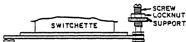
Fig. 2. Switchette adjustment, view from shaft end
