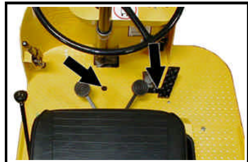
Spring adjuster access locations
