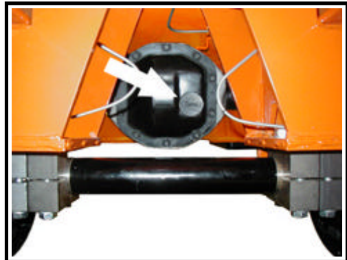
Fill plug viewed from the rear of the vehicle
