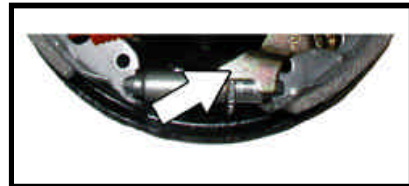
Close up of adjuster with brake drum removed. Arrow depicts the indexing lever.
