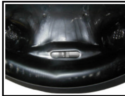
Star wheel seen through the access hole after the plug is removed
