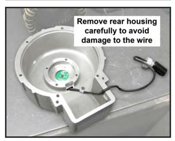
8: Using a soft face hammer tap on the rear motor housing (4) to separate it from the stator (2).
