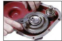
Idler Gear Circlip
