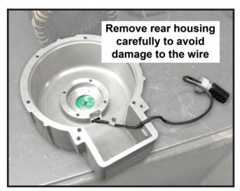
8: Using a soft face hammer tap on the rear motor housing (4) to separate it from the stator (2).
