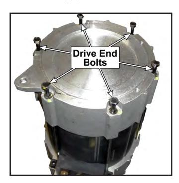
6: Using a soft face hammer, gently tap on the front motor housing (3) to remove.
