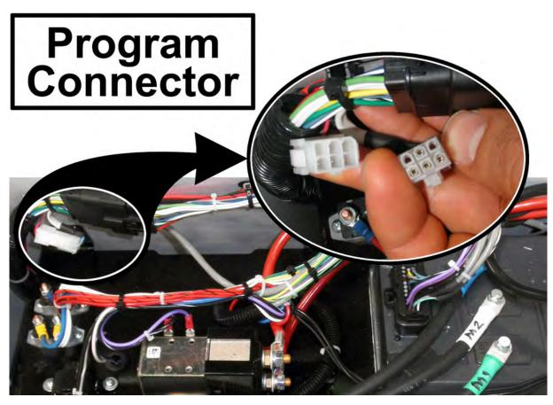
Program Connector is located under the rear deckboard on the Motor Speed Control Panel
