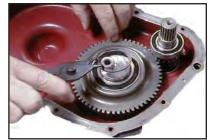
Idler Gear Circlip
