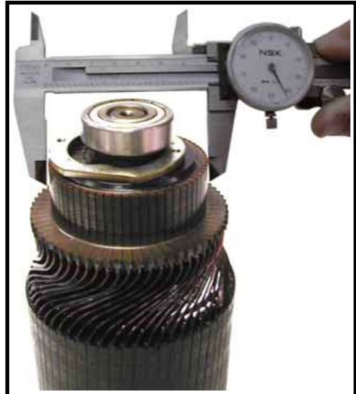
Example of freshly cut commutator
