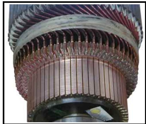
Example of freshly cut commutator
