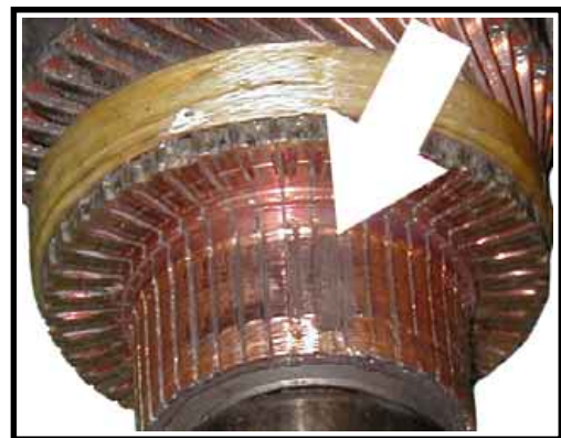
Typical burn mark on a shorted armature
