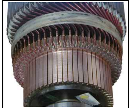
Example of freshly cut commutator
