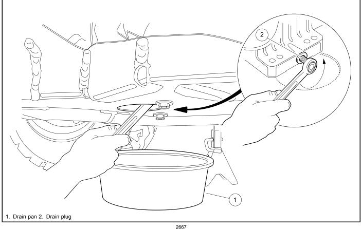
Figure 36 Engine Oil Drain Plug and Pan
