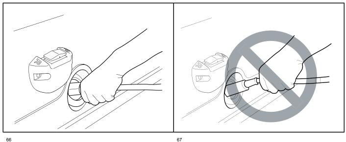
Figure 32 Correct Insertion of Charger DC Plug
