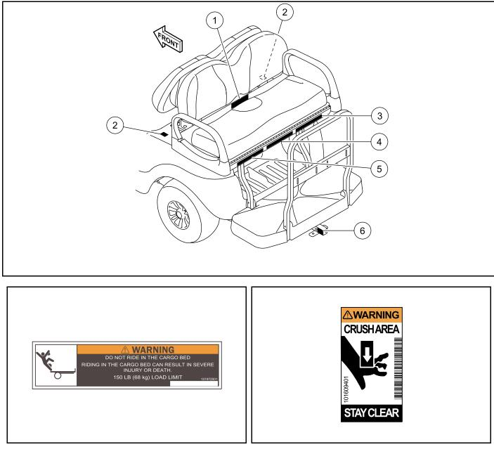
1. Decal, Box Bed Warning (P/N 101972001) 2. Decal, Crush Area Warning (P/N 101609401)
