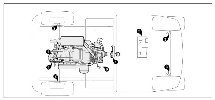
3117 Figure 26 Lubrication Points – Gasoline Vehicles
