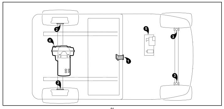
Figure 25 Lubrication Points – Electric Vehicles
