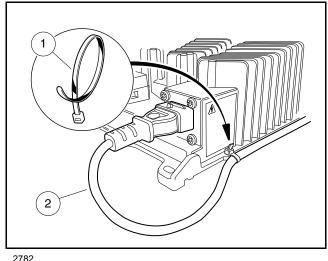
Figure 29 AC Cord Strain Relief and Drip Loop
