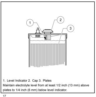
Figure 27 Battery Electrolyte Level
