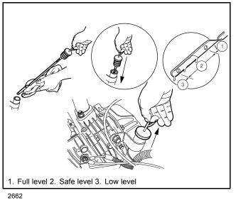
Figure 35 Engine Oil Level Check
