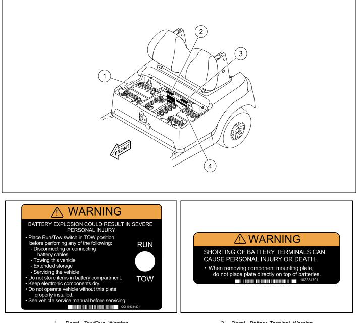
1. Decal, Tow/Run Warning (P/N 103384801) 2. Decal, Battery Terminal Warning (P/N 103384701)
