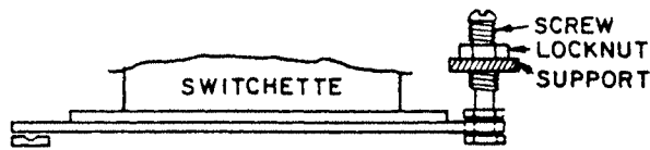
Fig. 2. Switchette adjustment, view from shaft end
