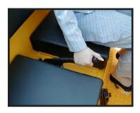
The parking brake is actuated with a hand lever, which is located between the driver and passenger seats. To set the parking brake, push down on the brake pedal and pull the lever up until it locks. To release the park brake, depress the foot brake pedal, pull up on the park brake handle, push the release button, and lower the handle.
