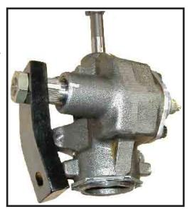
Steering Gear with Pitman Arm
