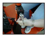
The hazard light switch is located on the left side of the steering column. The switch is a small tab. To activate the hazard lights, pull the tab out. To turn the hazard lights off, push forward or pull back the directional signal lever.
