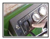
The accessory switch is located on the left side of the instrument panel and to the right of the headlight switch. Push the top of the switch to turn on an accessory. Push the bottom of switch to turn off the accessory. The accessory can be turned on with the key switch in the "OFF" position. If a vehicle is equipped with windshield wipers and one or more accessories, the windshield wipers are controlled from this switch. Other accessories are controlled from the auxiliary switch.
