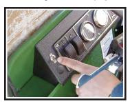
The auxiliary switch is located on the left side of the instrument panel and to the left of the headlight switch. Push the switch up to turn on an accessory. Push the switch down to turn off the accessory. The accessory can be turned on with the key switch in the "OFF" position. If a vehicle is equipped with windshield wipers and one or more accessories, the auxiliary switch will control the other accessories.
