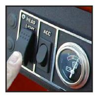
The headlight switch is located on the far left side of the instrument panel. Push the top of the switch to turn the lighs on. Push the bottom of the switch to turn the light off.
