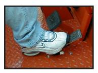
The accelerator pedal is located to the right of the brake pedal. It controls the speed of the vehicle and operates similar to the accelerator pedal in an automobile. Depress the pedal to increase speed and release the pedal to decrease speed.
