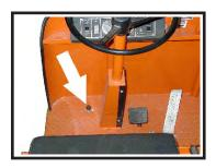
The horn switch is located to the left of the steering column. Depress the switch with your left foot to sound the horn, release it to turn it off.
