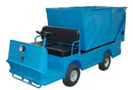
B 2-48-36 Equipped with optional hydraulic dump bed
