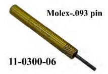
Molex # 11-300-06: Pin Removing Tool Removes 0.093 diameter pins from Molex rectangular harness connectors. Not available from Taylor-Dunn. Purchase from any local electronics distributor.
