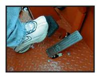
The foot brake pedal, is located to the right of the steering column, it is for operation with the right foot only. It works similar to the brake in an automobile. Applying pressure to the brake pedal slows the vehicle according to the amount of pressure applied. Relieving pressure from the pedal releases the braking action.
