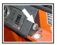
A key-switch, located on the right side of the instrument panel, turns on the vehicle. Rotate the key clockwise to turn the vehicle power on, counterclockwise to turn the vehicle power off.
