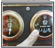
The hour meter is located to the right of the battery status indicator. It records the number of hours the vehicle has been in operation.
