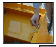
A switch located under the driver's seat disables the power to the vehicle when the driver leaves the seat. The driver must be seated for the vehicle to operate.
