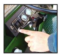
The turn signal lever is located on the left side of the steering column. Push the lever forward to activate the right turn signal and pull the lever back to activate the left turn signal.
