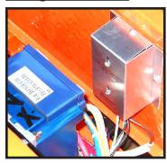
The charger interlock is designed to disable the vehicle from being driven while the AC charger cord is plugged into a functioning power source.
