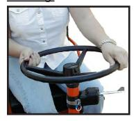
The steering wheel and steering system are similar to an automobile. To turn right, turn the steering wheel clockwise. To turn left, turn the steering wheel counter-clockwise.
