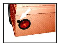
The reverse alarm is located in the electronics compartment mounted on the speed control panel or on the rear panel of the vehicle. The reverse alarm is activated when the Key switch is in the "ON" position and the Forward-Reverse switch is in the reverse position. The alarm makes a repeated audible sound.
