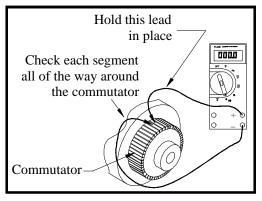
11. Measure the armature and field resistance (refer to Service Limits table at end of this section). If the armature of field resistance is not within specification then the motor must be repaired or replaced.
