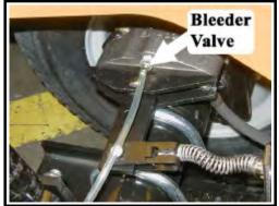
Bleeder valve with hose attached
