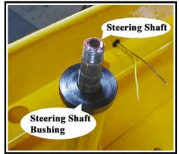
NOTE Most vehicle configurations will now allow the steering shaft to slide off of the steering gear input shaft and then back down out of the steering column. If there is not enough clearance for this procedure then the steering gear must be removed. Refer to **Replace the Steering Gear** for information regarding removing the steering gear.
