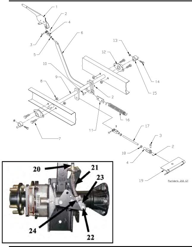
Brake linkage (parking brake), B 2-10
