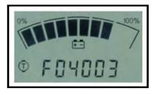
**Speed controller status:** The display will indicate a fault code whenever the control system logic detects a problem with the control system. A fault code is being displayed whenever the Fault Code Indicator (the letter 'F') is visible at the left of the numeric display. Refer to the fault code table in this section for a summery description of the fault codes.
