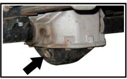
8. If no oil comes out, then lift the side of the vehicle with the level plug and add 11-ounces of oil through the level plug hole. See the illustration below.
