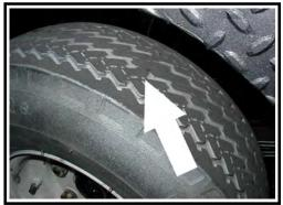
8. Inspect for uneven tire wear on the front tires. Uneven tire wear could be a result of an improperly inflated tire or a misaligned or damaged front end.
