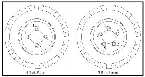
Pattern for tightening the wheel nuts
