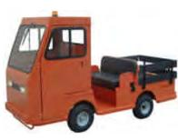
B2-48 with Steel Cab, Foldaway 4-Passenger Seat and Stake Sides
