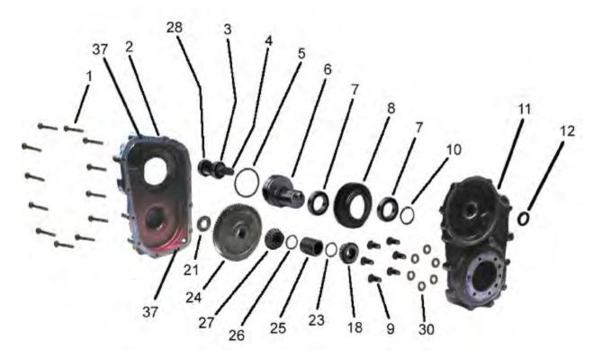
Note 1: Spacer 23 is available in increments of .05mm starting at 3.9mm. 3.9mm spacer is part number GT-3287213. Add 10 to the part number for every 0.05mm over 3.9. For example, if 4.55mm is needed: 4.55-3.9 = .65mm over, 0.65/.05 = 13, 13\*10 = 130. Part number for 4.5mm spacer is 3287213+130 = 3287343.
