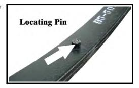
8. Install the four u-bolts so that the u-bolt nuts are tight enough to hold the springs on the locating pins but not so tight as to keep the springs from moving.
