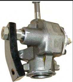
Steering Gear with Pitman Arm
