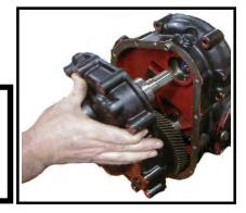
12. Remove the circlip from the idler gear.
