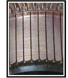
Properly undercut and cleaned commutator segments
