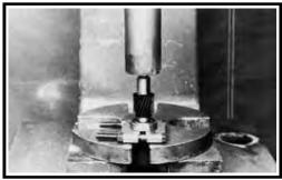
3. Insert new o-rings into both sides of the intermediate shaft bore, the input shaft bore and the intermediate shafts.
