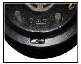
Brake drum with adjusting slot aligned with star wheel
