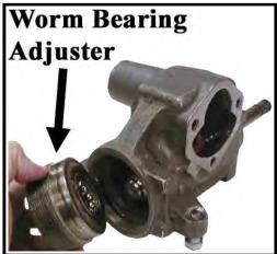
16. Once the adjustments are completed, make sure that the locking ring and jam nut are tight.
