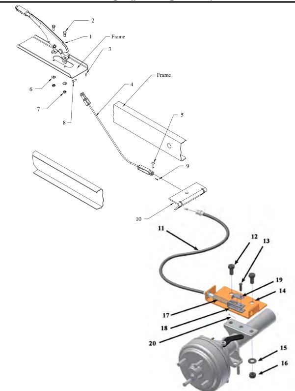
Brake linkage (parking brake), B 2-00
