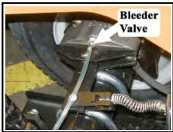
Bleeder valve with hose attached
