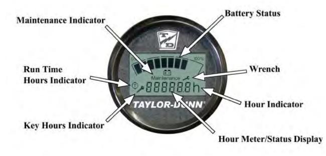
The Smart View Display (SVD) functions as a Battery Status Indicator (BSI), Hour Meter (HM), speed controller status monitor, and as an optional maintenance monitor feature. The operation of each of these functions is described below. The Smart View is optional for the B 2-00.
