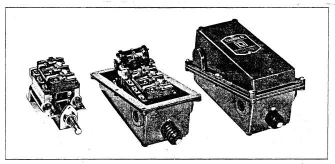
**APPLICATION** — The accelerating master switch for truck control is a manually operated pilot device to control magnetic contactors, which in turn, control the traction motor of an electric truck. It provides either three or four individual speeds and may have time delay acceleration and plugging control.
