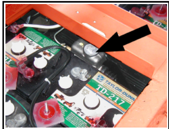
Dana 36 and 48v, Ford 36v. The master cylinder is located in between the batteries
