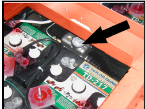
The master cylinder is located in between the batteries
