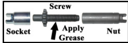
Brake Adjuster Assembly
