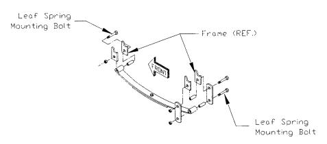
Drive Assembly: The drive assembly is mounted to the frame by the leaf spring
