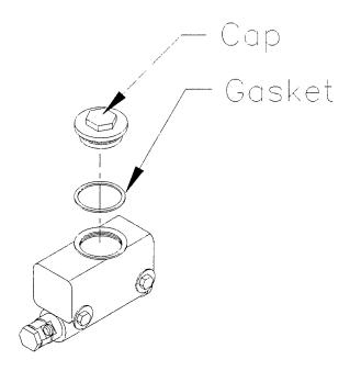
Brake Figure 7: Filling Master Cylinder
