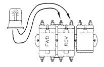
If the light did not come on at all, then check all power wiring for opens. Stop here and repair the problem.
