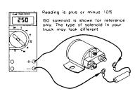
Measuring the Resistance of ISO Solenoid Resistor: The resistor is test with the meter set to ohms. The correct reading is 250 ohms +/- 10- percent.
