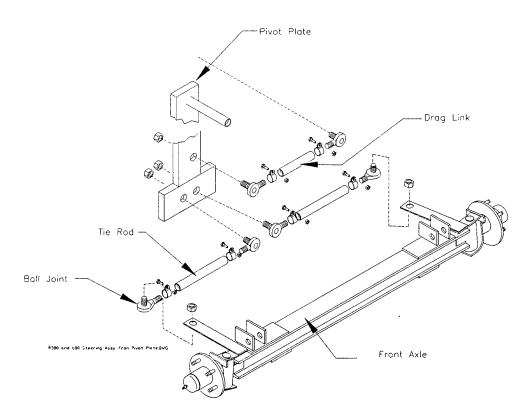
Front Axle Figure 8: Steering Components
