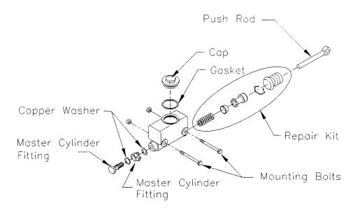
Brake Figure 6: Master Cylinder
