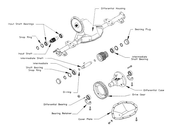
Exploded view of the differential assembly: This view shows the parts contained with in the differential. Part numbers are available in the Illustrated Parts section of this manual.
