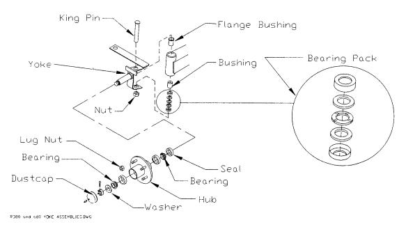
Front Axle Figure 4: Yoke Assembly
