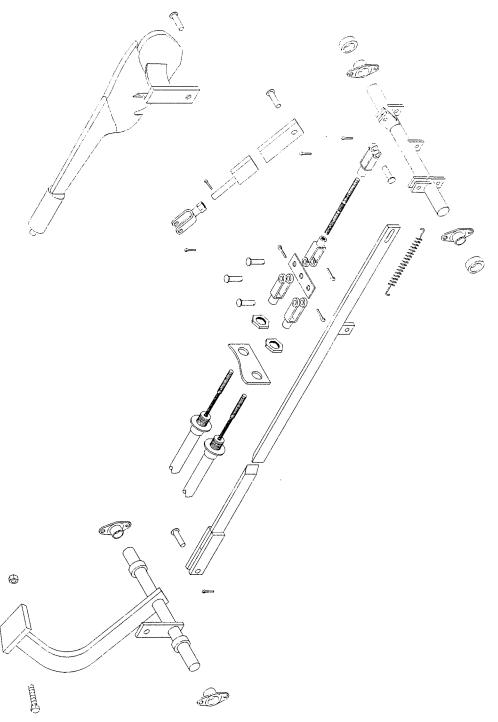
Park Brake Figure 9: Exploded View of Parking Brake
