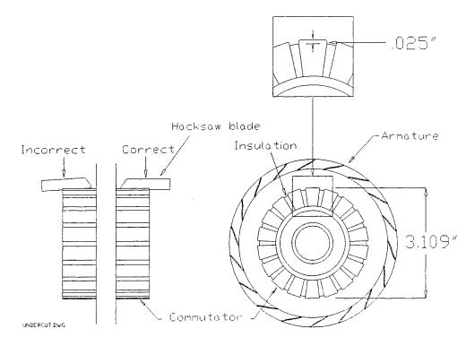
Drive Motor Figure 1: Under Cut
