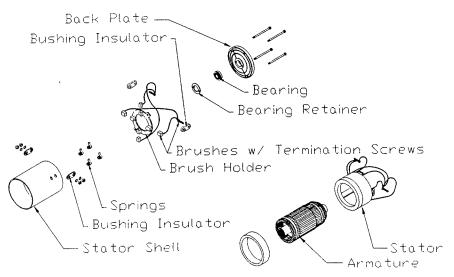
Exploded View of the 70-049-05 Motor.
