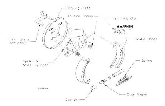
The Star Wheel and The Adjusting Slot on the brake drum must be lined up in order to make adjusments
