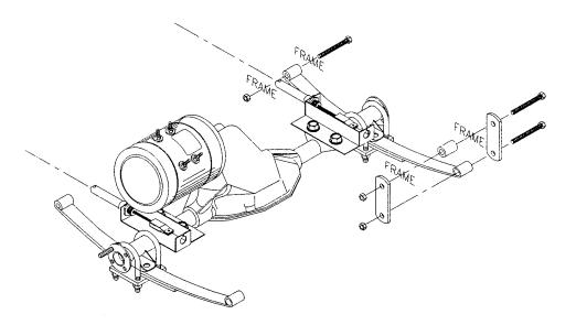
Complete Drive Assembly Less Motor: Shown is the complete drive assembly without the motor.
