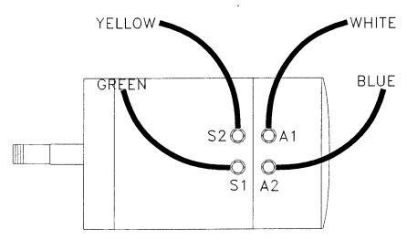
Typical wire connections on motor: In this figure we show the wire connections to the motor and their colors. Be sure to label each of the wires with their correct locations before removing them from the motor.
