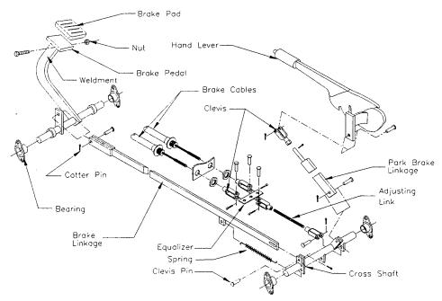
Brake Figure 2: Mechanical Brake Linkage
