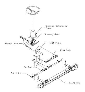
Front Axle Figure 12: Complete Steering Assembly
