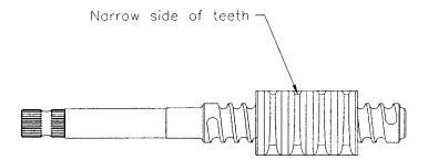
Front Axle Figure14: Worm Shaft
