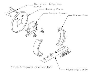
Brake Figure 1: Mechanical Brake
