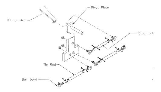
Front Axle Figure16: Ball Joint and Drag Link
