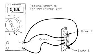
5) Reconnect the lead to the diode.
