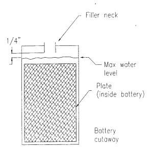
Battery Fill Level: This figure show the proper fill
