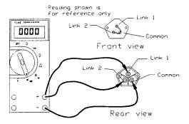
3) Disconnect one lead from the capacitor. Test the capacitor using the capacitor test function of your meter. It is a 6-microfarad capacitor. If the capacitor is bad, it must be replaced. Stop here and repair the problem.
