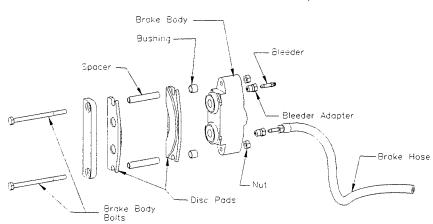
Front Hydraulic Disc Brake Body.
