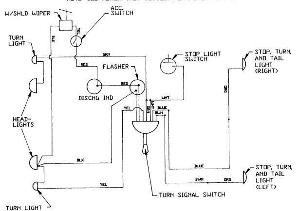
TURN SIGNAL AND WIPER MOTOR WIRING DIAGRAM
