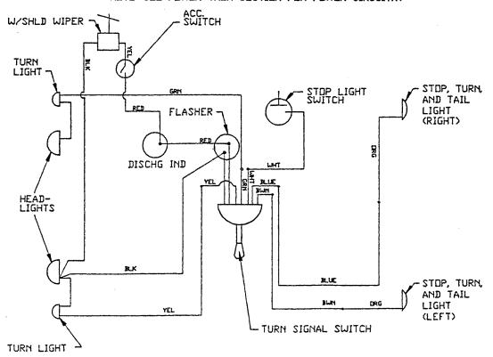
TURN SIGNAL AND WIPER MOTOR WIRING DIAGRAM
