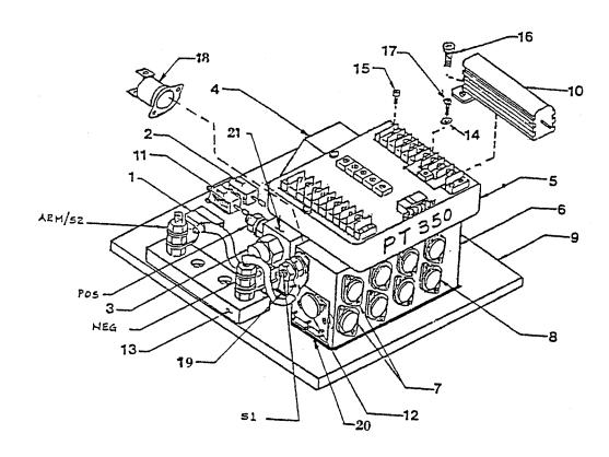
$$62\text{-}\emptyset35\text{-}\emptyset\emptyset$$  PWR-TRON 350 SPEED CONTROLLER AND PARTS LIST
