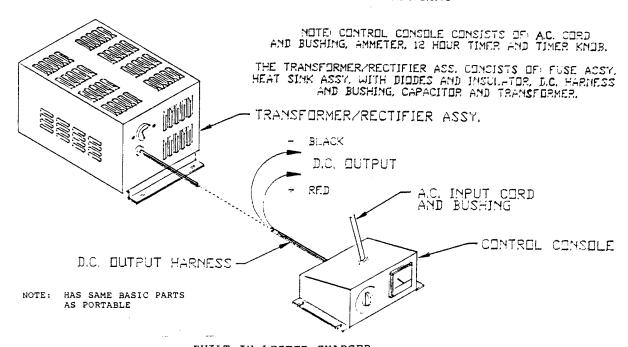
BUILT-IN LESTER CHARGER (TYP!CAL) FOR COMPONENT IDENTIFICATION SEE PARTS LIST FOR BUILT-IN CHARGERS
