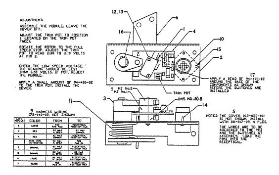
ACCELERATOR (SOLID STATE) MODULE (COVER NOT SHOWN) 62-033-00
