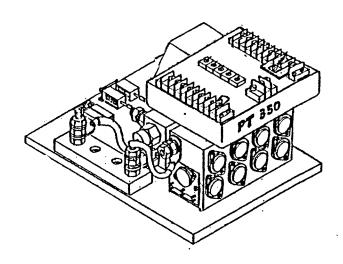
24 OR 36 VOLTS RECOMMENDED FOR USE UP TO 10 HP MOTORS (INTERMITTENT)
