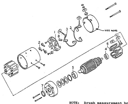
Brush measurement holes (2). With new brushes a 1/16" drill rod can be inserted approximately.780" into the brush measurement holes. Brushes should be replaced when rod can be inserted 1.560" into hole. This leaves approximately 1/8" wear remaining.
