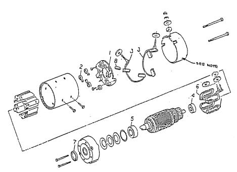
NOTE: Brush measurement holes (2). With new brushes a 1/16" drill rod can be inserted approximately.780" into the brush measurement holes. Brushes should be replaced when rod can be inserted 1.560" into hole. This leaves approximately 1/8" wear remaining.
