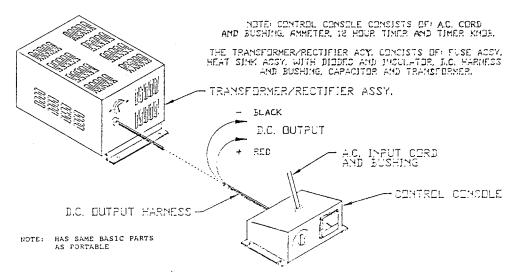
BUILT-IN LESTER CHARGER (TYPICAL) FOR COMPONENT IDENTIFICATION SEE PARTS LIST FOR BUILT-IN CHARGERS
