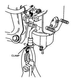
Carburetor Figure 1: Removing Fuel Line
