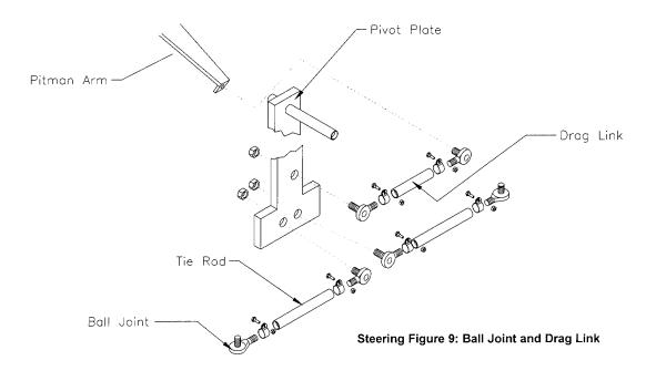
Replace Drag Link, Tie Rods and Ball Joints
