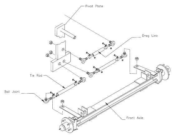
In this segment, we will discuss how to remove and replace these parts from the steering system, with the exception of removing the steering wheel. The steering system has been designed for the easy removal and replacement of parts.
