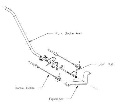
Brake Figure 4: Park Brake Cable Linkage
