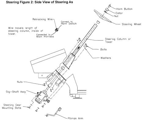
To Remove the Steering Column or Tower
