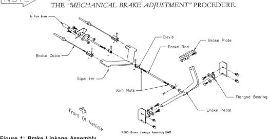
Brake Figure 1: Brake Linkage Assembly
