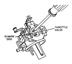
Carburetor Figure 11: Throttle Valve ID Marks
