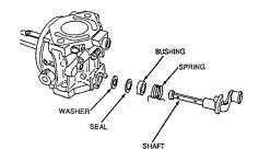
Carburetor Figure 10: Remove Choke Shaft and Air Jet
