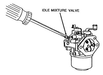
Carburetor Figure 13: Needle Valve Adjustment
