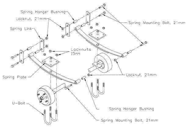
**Rear Suspension Figure 1: Rear Suspension**
