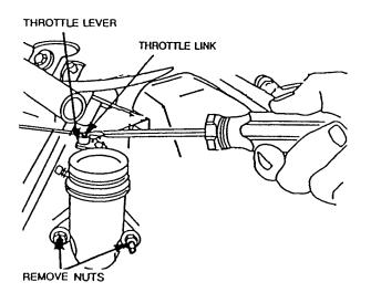
Carburetor Figure 4: Removing the Gonenor Link and Intake Elbow
