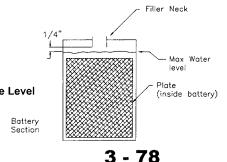
Battery Figure 2: Electrolyte Level
