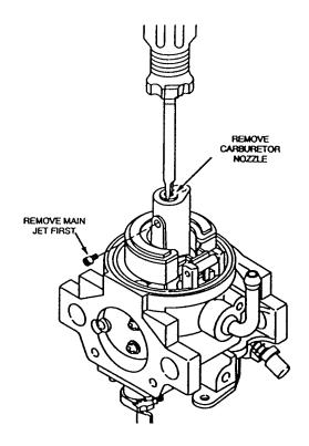
Carburetor Figure 5: Remove Main Jet
