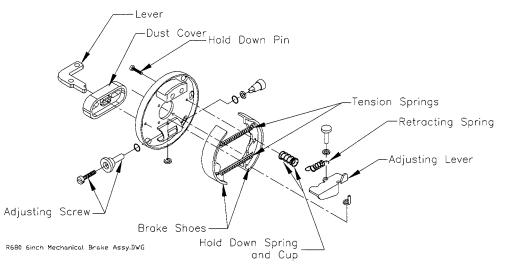
Brake Figure 2: Brake Shoe Replacement
