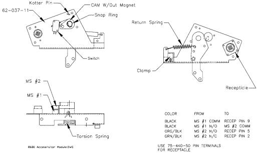
Accel Figure 2: Accelerator Module
