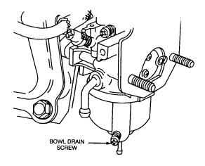
**Carburetor Figure 2: Draining Carburetor**
