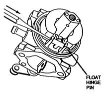
**Carburetor Figure 6: Remove Float**
