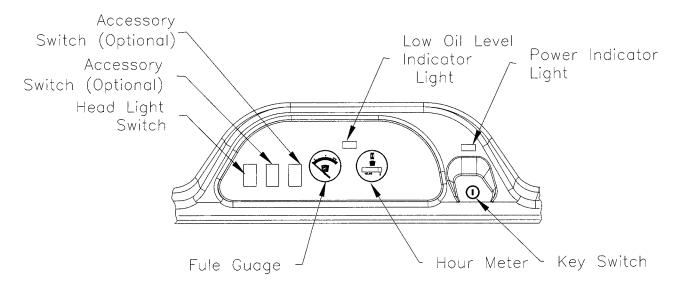
Figure 2-1: Dash Panel with Controls
