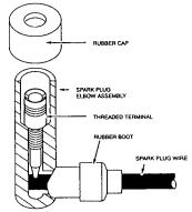
Engine Figure 2: Spark Plug Terminal Wire
