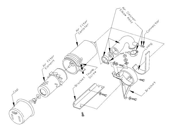
Engine Figure 10: Air Filter Assembly
