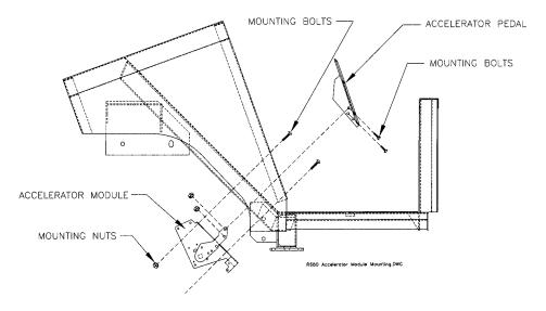
Accel Figure 1: Acclerator Module Mounting
