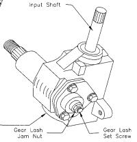
how far the input shaft is turned before the output shaft begins to move. Adjusting for gear lash is a maintenance function and should be included in any maintenance schedule.
