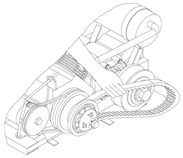
Engine Figure 9: Removing the Drive Belt
