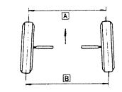
A Center-to-center at front side tire tread. B Center-to-center at rear side tire tread.
