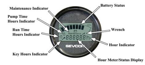
The Smart View Display (SVD) functions as a Battery Status Indicator (BSI), Hour Meter (HM), speed controller status monitor, and as an optional maintenance monitor feature. The operation of each of these functions is described below.
