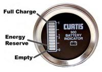
flashing the batteries are empty and the truck should be taken out of service and charged to avoid damaging the batteries. The BSI will reset to fully charged only after a complete charge cycle is completed. A complete charge cycle is defined as battery voltage exceeding 2.35 volts per cell for a minimum of 6 minutes.
